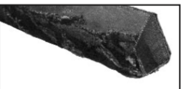
Cover Fabric Rupture Cause: Fabric covering ruptured during installation due to belt being pried over belt sheave. Remedy: Proper installation of belts.
