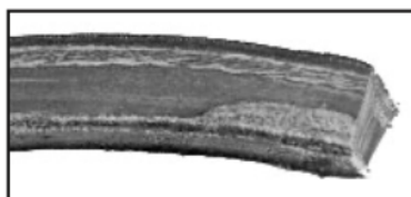
Worn Side Pattern Cause: Worn or misaligned sheaves. Remedy: Retension drive to stop slipping, realign sheaves (replace if needed), replace belt if incorrect size.
