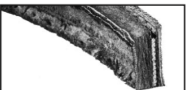
Oil Deterioration Cause: Rubber softened by excessive oil exposure, causing deterioration. Remedy: Splash guards to protect drive against oil.
