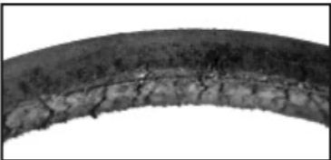
Weathering or "Crazing" Cause: Belt drive elements, as well as aggravation by small sheaves. Remedy: Check tension, provide drive protection and replace belt(s).
